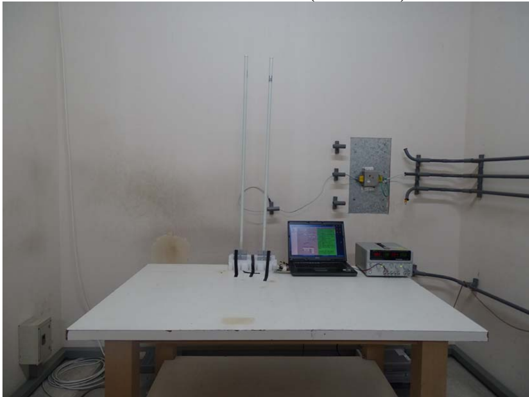
Front View of Conducted Test (Omni Antenna)
