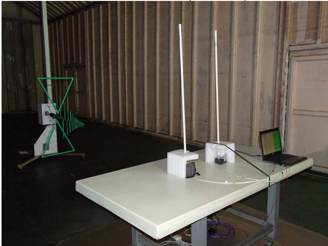
Front View of Radiated Test (Omni Antenna)
