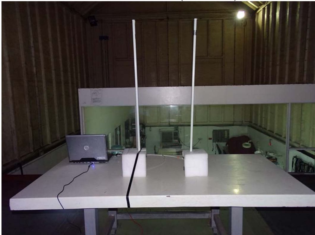
Back View of Radiated Test (Omni Antenna)
