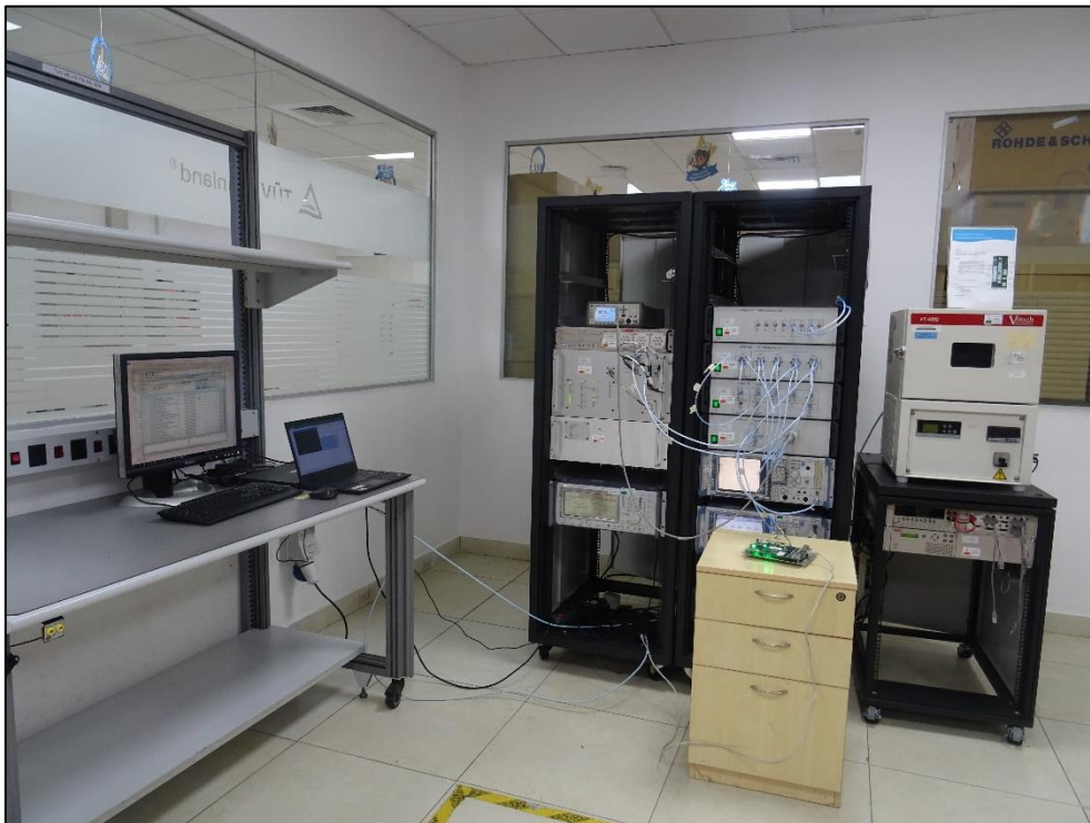
Conducted Test Setup Photo
