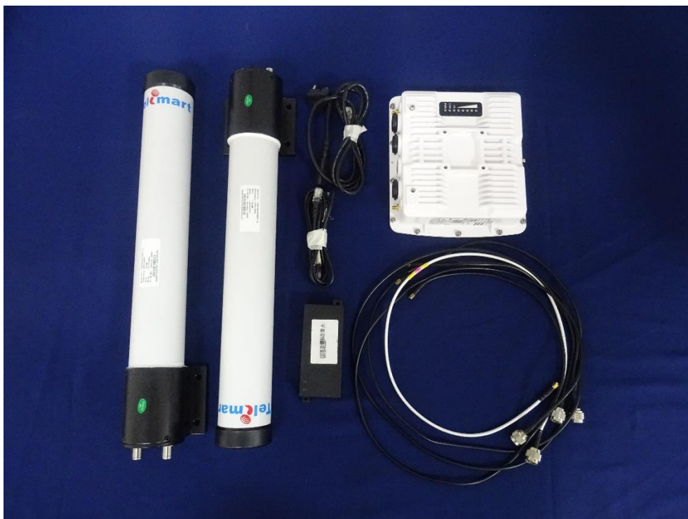
Photo 6: EUT With Omni Antenna
