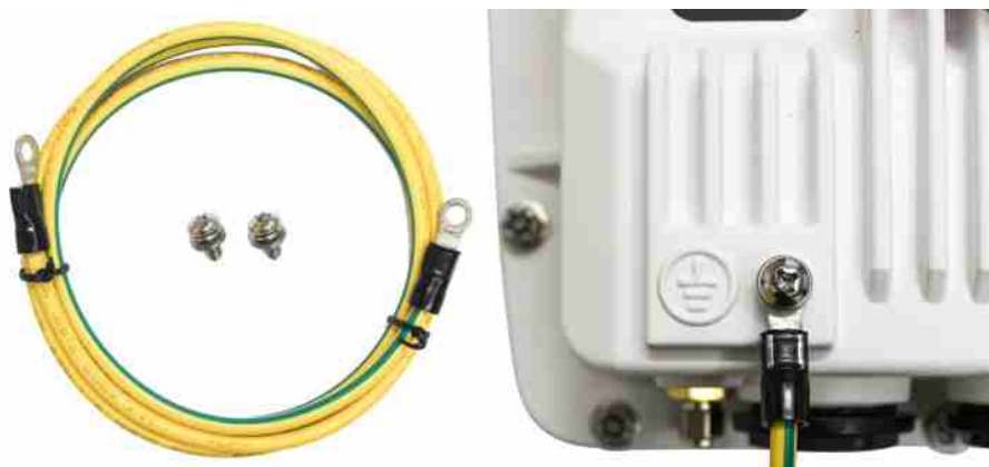
Figure 4-7 Ground the Device
