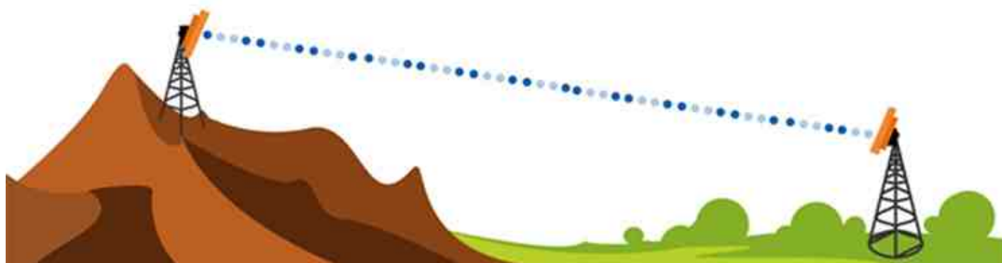
Figure 8-2 Typical installation showing device/antenna tilt angle
