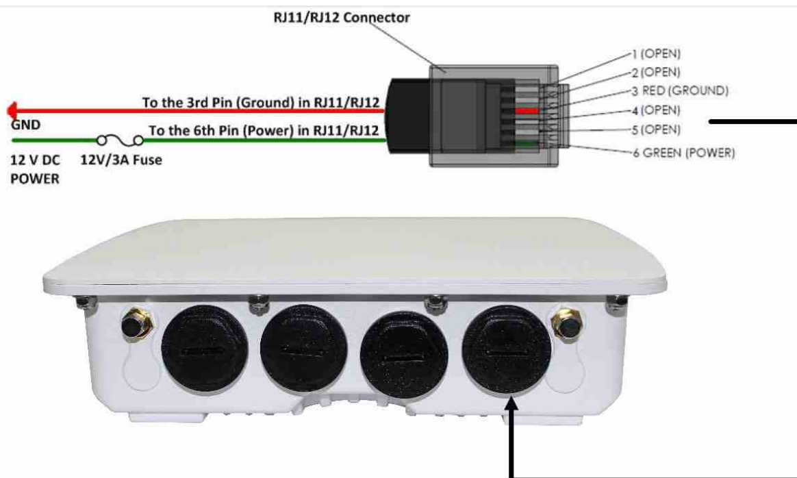
Figure 3-3 Powering the device through Access Port using 12 V DC Power Supply
