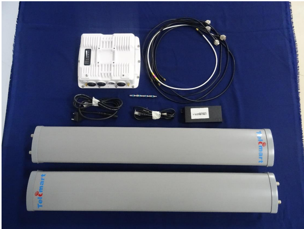
Photo 7: EUT With Sector Antenna
