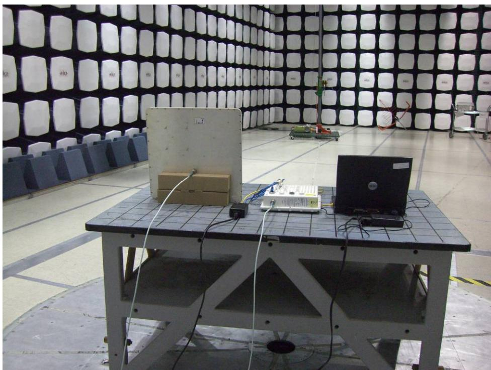
**10.7 Radiated Emissions – Front View (Omni - Directional Antenna 10.0dBd Gain)**
