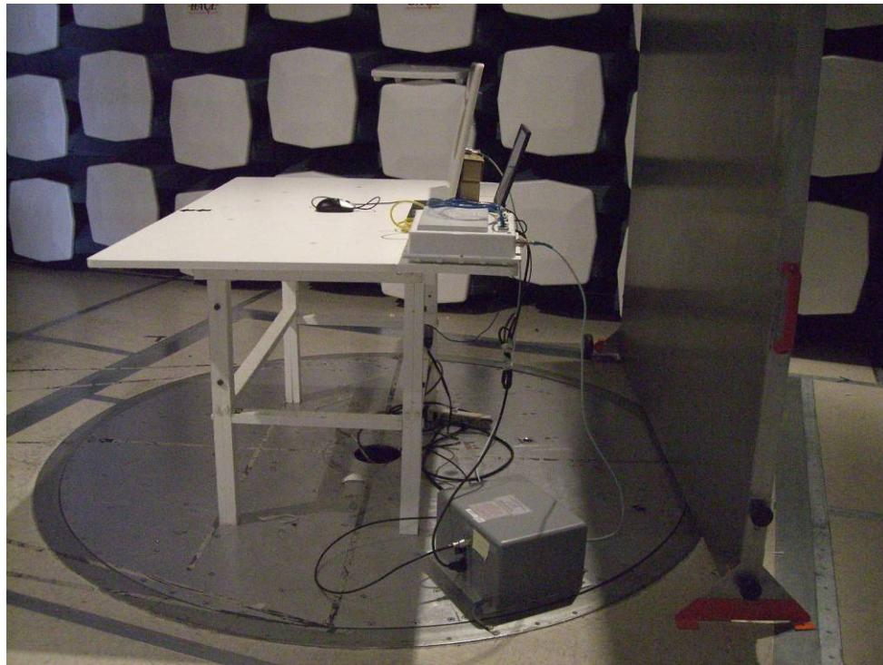
**10.3 Radiated Emissions – Front View (Sector Panel Antenna 17dBD Gain)**
