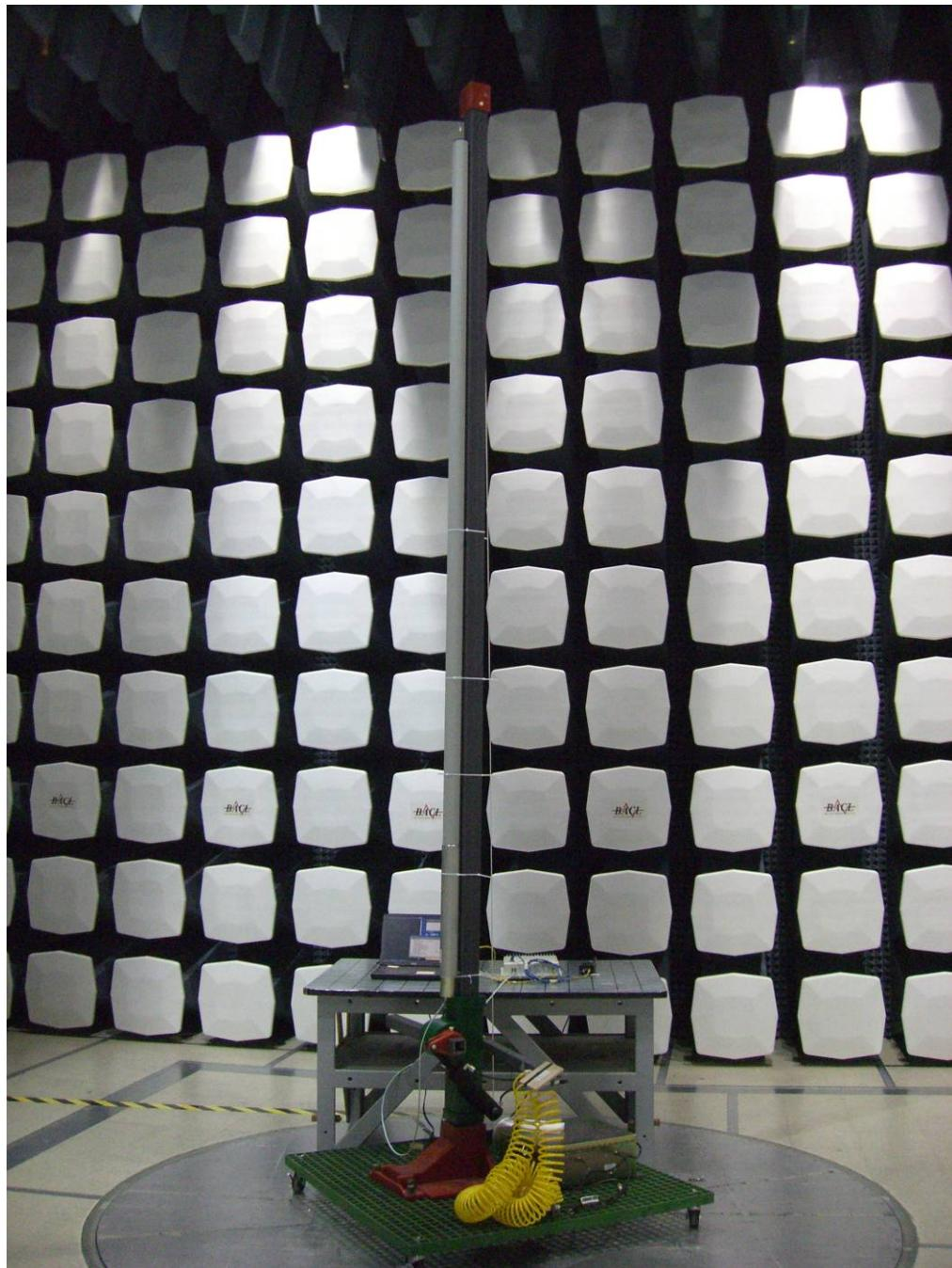
**10.8 Radiated Emissions – Back View (Omni - Directional Antenna 10.0dBd Gain)**
