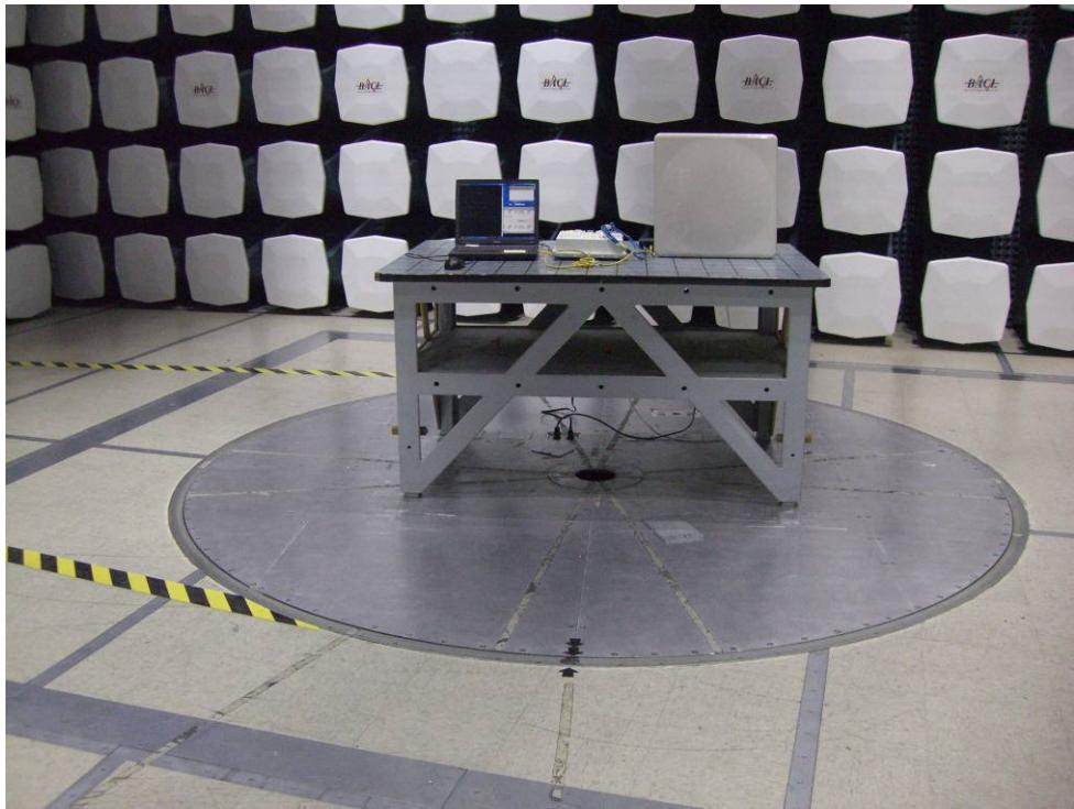
**10.6 Radiated Emissions – Back View (Flat Panel Directional Antenna 12.5dBi Gain)**
