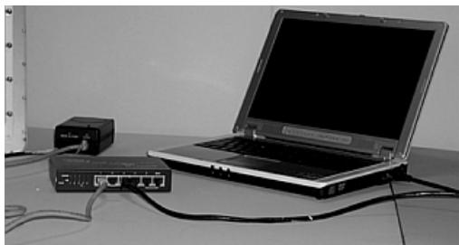
**Note:** If you are connecting the PC directly to the unit, you must use a crossover Ethernet cable between the network interface card in the PC and the RJ45 "Data In" port on the power injector.
