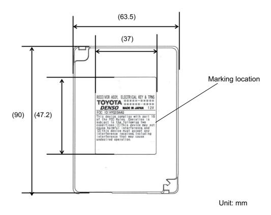
Fig. Marking location and Appearance of Receiver
