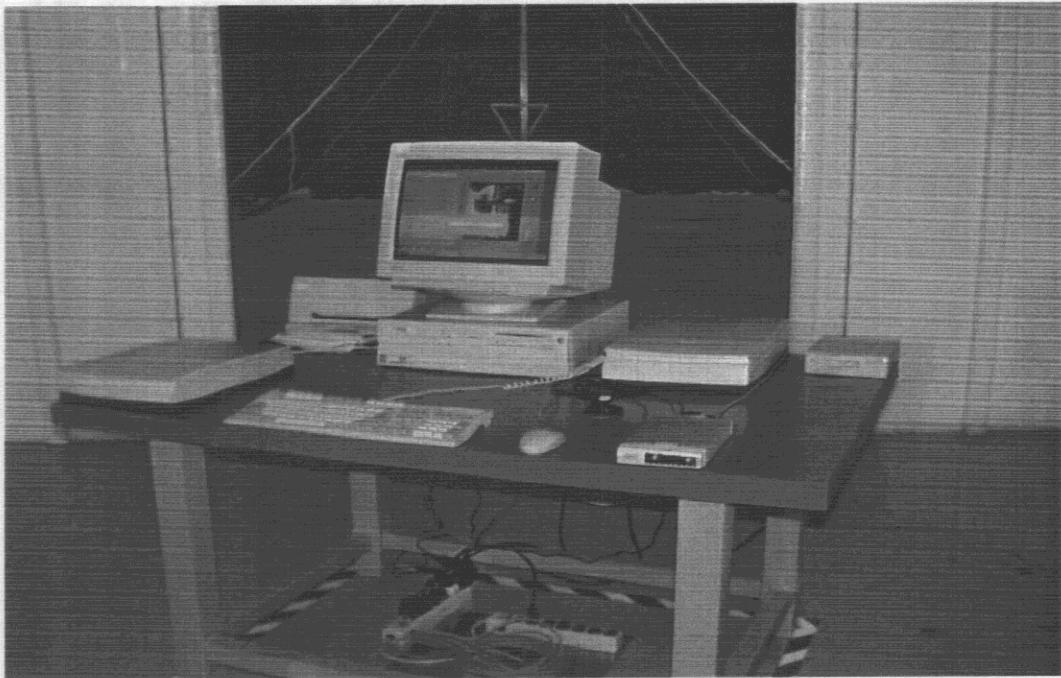
**8. BACK VIEW OF RADIATED TEST ( Worst Case Test Setup, mode 2)**
