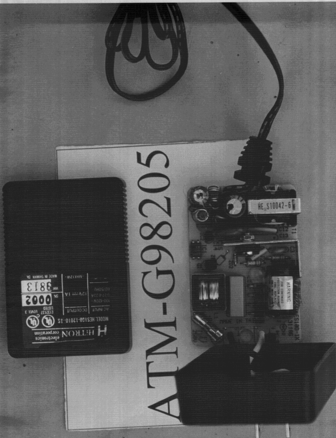
Figure 12 Cover & PCB View of Power Adapter
