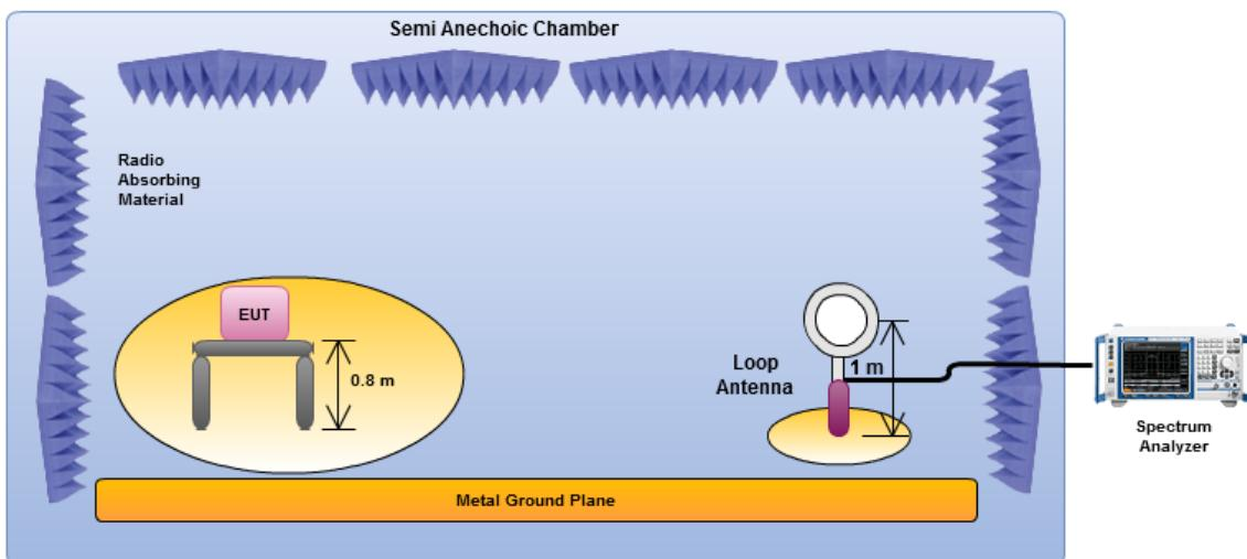
Magnetic field tests shall be performed in the frequency range of 9 kHz to 30 MHz using a calibrated loop antenna. The center of the loop shall be 1 m above the ground.
