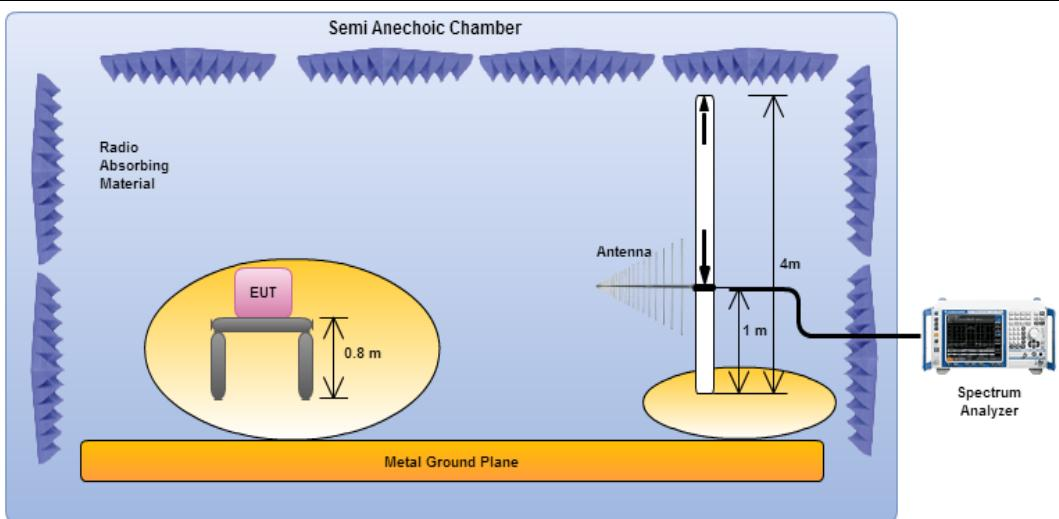
Electric field tests shall be performed in the frequency range of 30 MHz to 1000 MHz using a calibrated bi-log antenna. the antenna height shall be varied from 1 m to 4 m.
