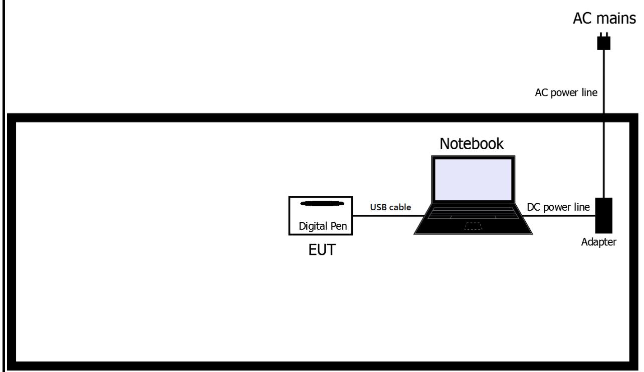
Test Setup Diagram - Radiated Emission Test
