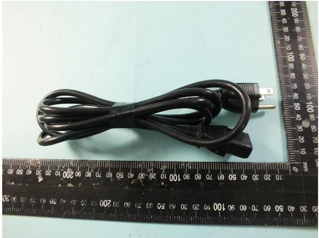
AC Power Cable (FCC)
