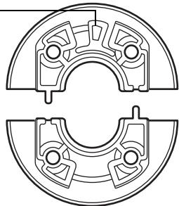
When correctly placed, the bearing stopper will shift smoothly from side to side within the stopper groove. The stopper will also sit flush with the rear hub surface.
