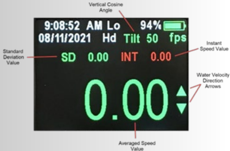
Figure 4.2.4 Digital display operation with status indicator icons.
