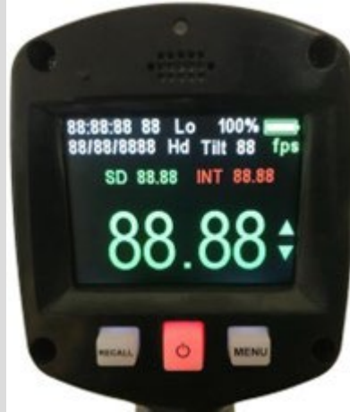
Figure 4.1a Faceplate ( Display and Control Buttons)
