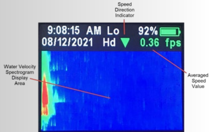
Figure 4.2.6 Mode 2 Spectrogram display with status indicator icons.
