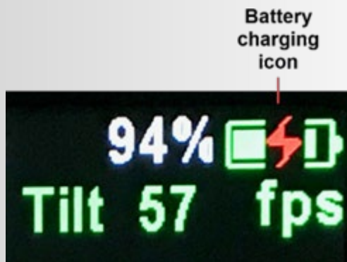
Figure 3.3c Battery and charging status while SVR 3D is ON and charging
