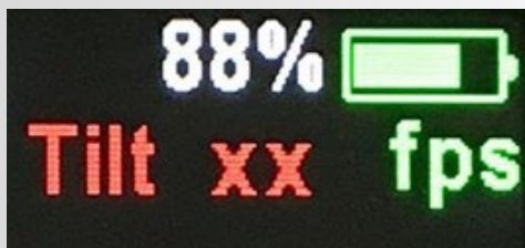
Figure 7.1b The display when the vertical (pitch-down) angle exceeds 60°
