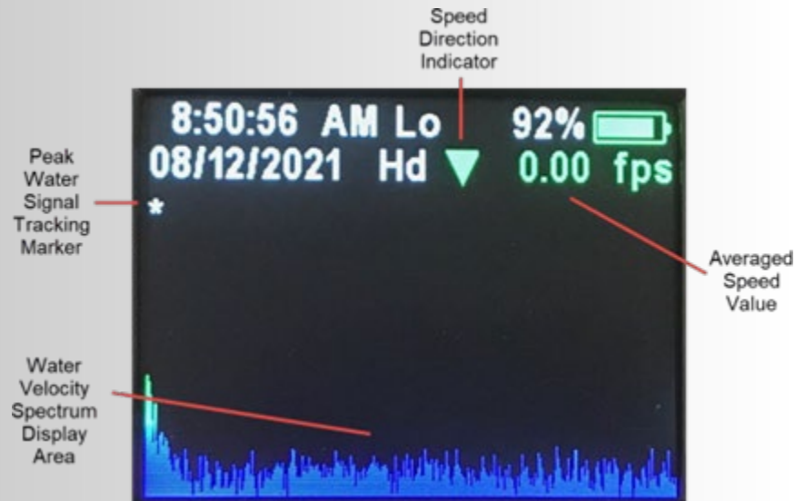
Figure 4.2.5 Mode 1 Spectrum display with status indicator icons.
