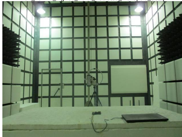
Part 15.247 ZigBee_Port2 Radiated Setup
