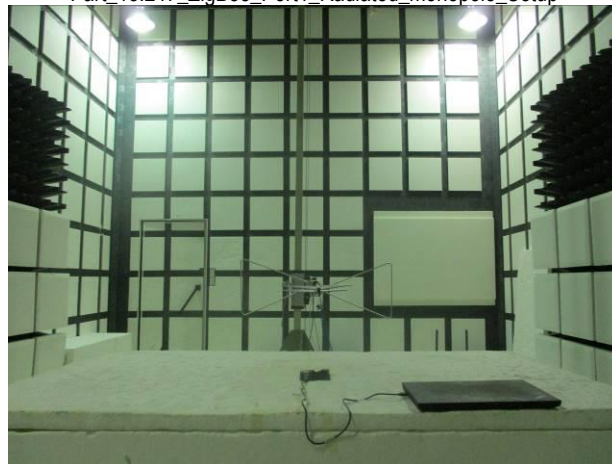
Part 15.247 ZigBee_Port1 Radiated monopole Setup
