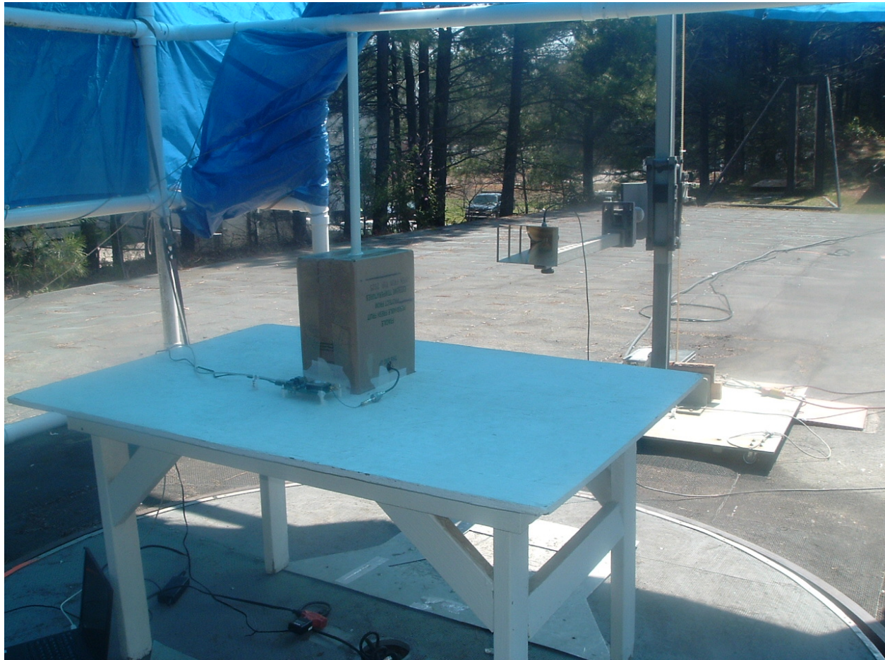
Photo 6. Above 1GHz Test setup at 1 meter
