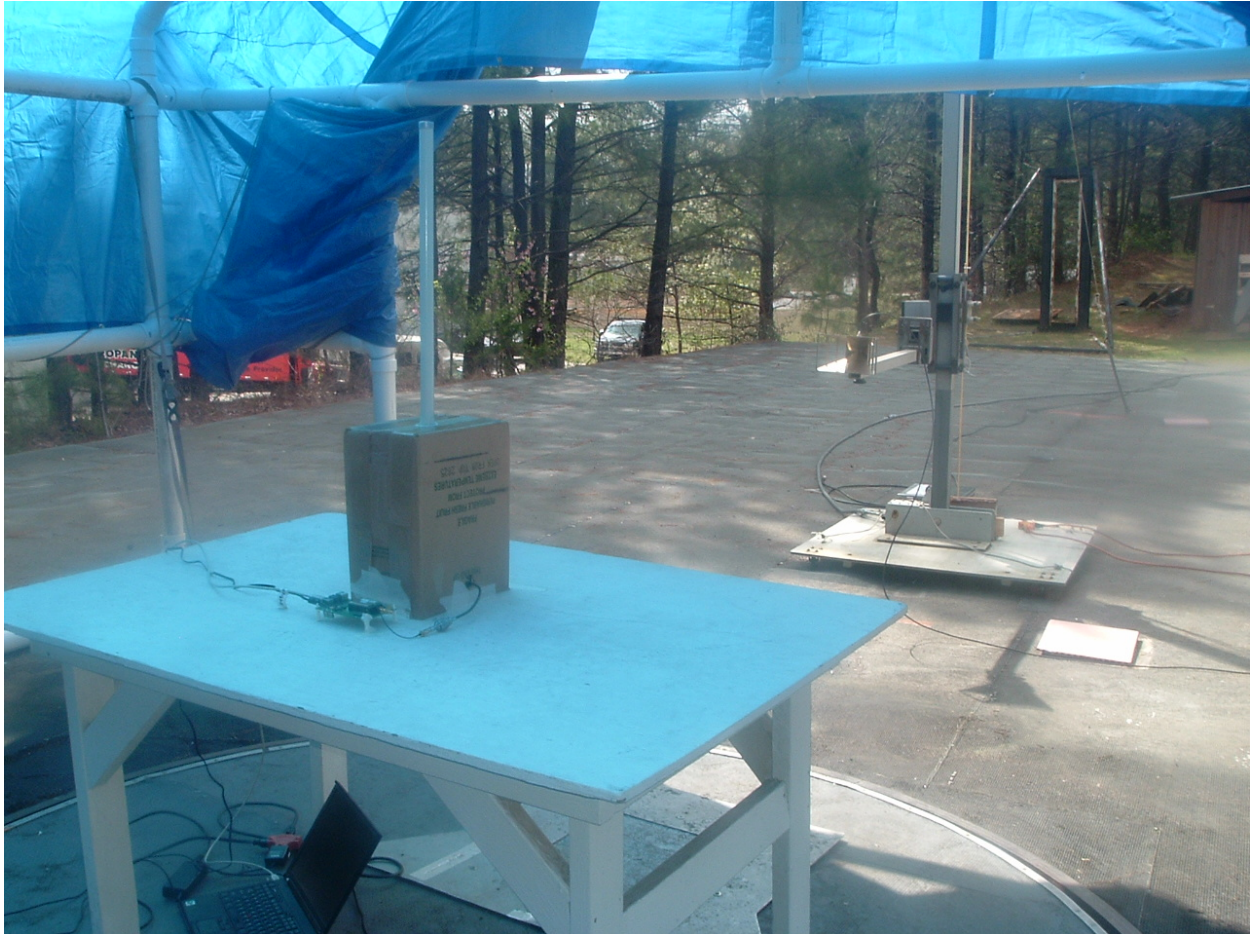
Photo 5. Above 1GHz Test setup at 3 meter
