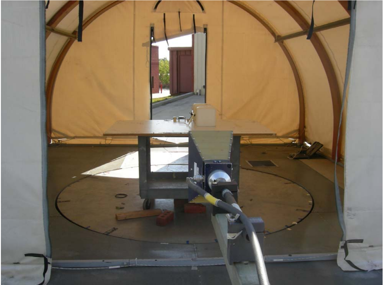
Figure 2: Radiated Emissions Test Set Up – Yagi Antenna
