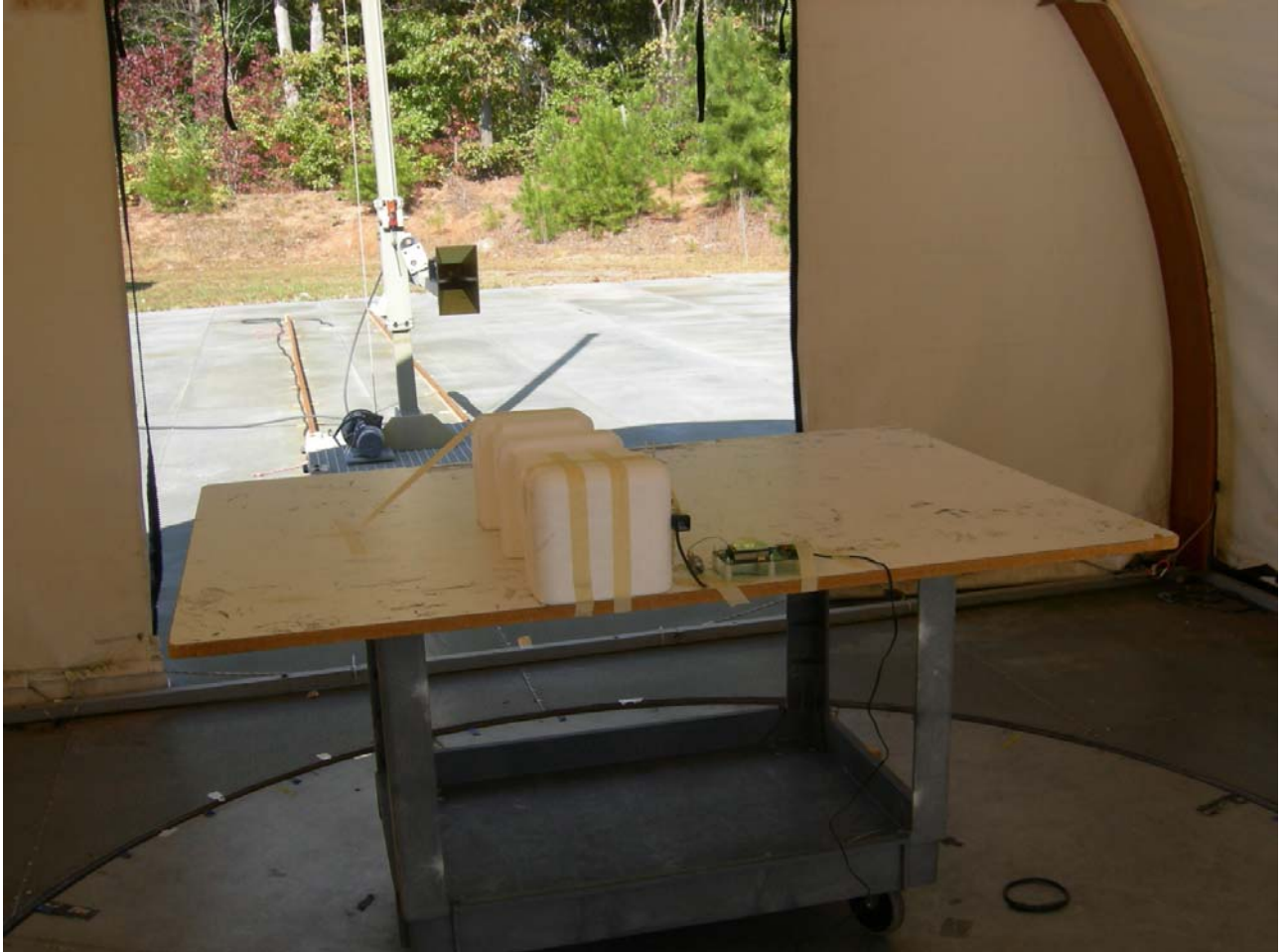
Figure 1: Radiated Emissions Test Set Up – Yagi Antenna
