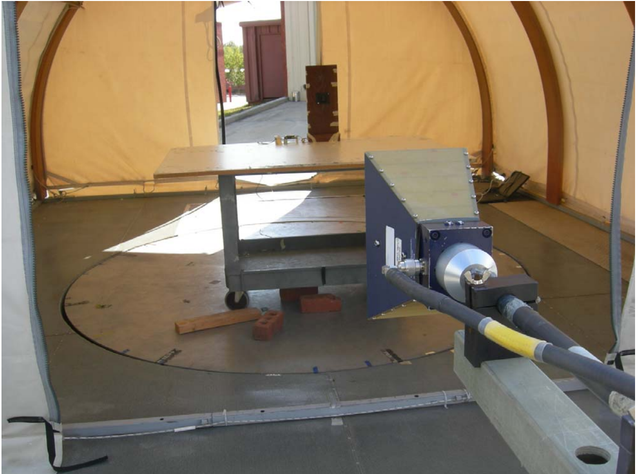
Figure 5: Radiated Emissions Test Set Up – Dipole Antenna
