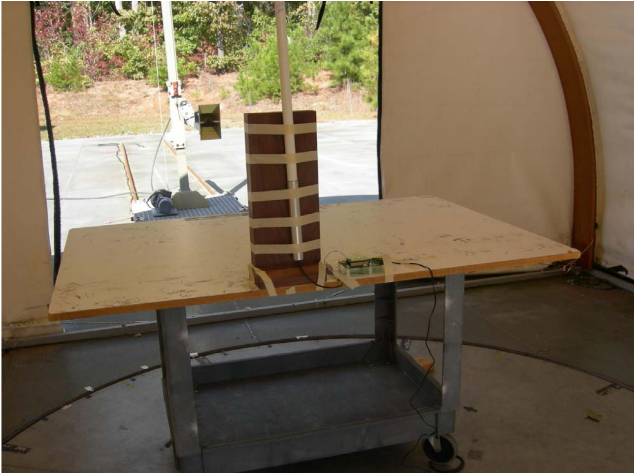
Figure 4: Radiated Emissions Test Set Up – Dipole Antenna
