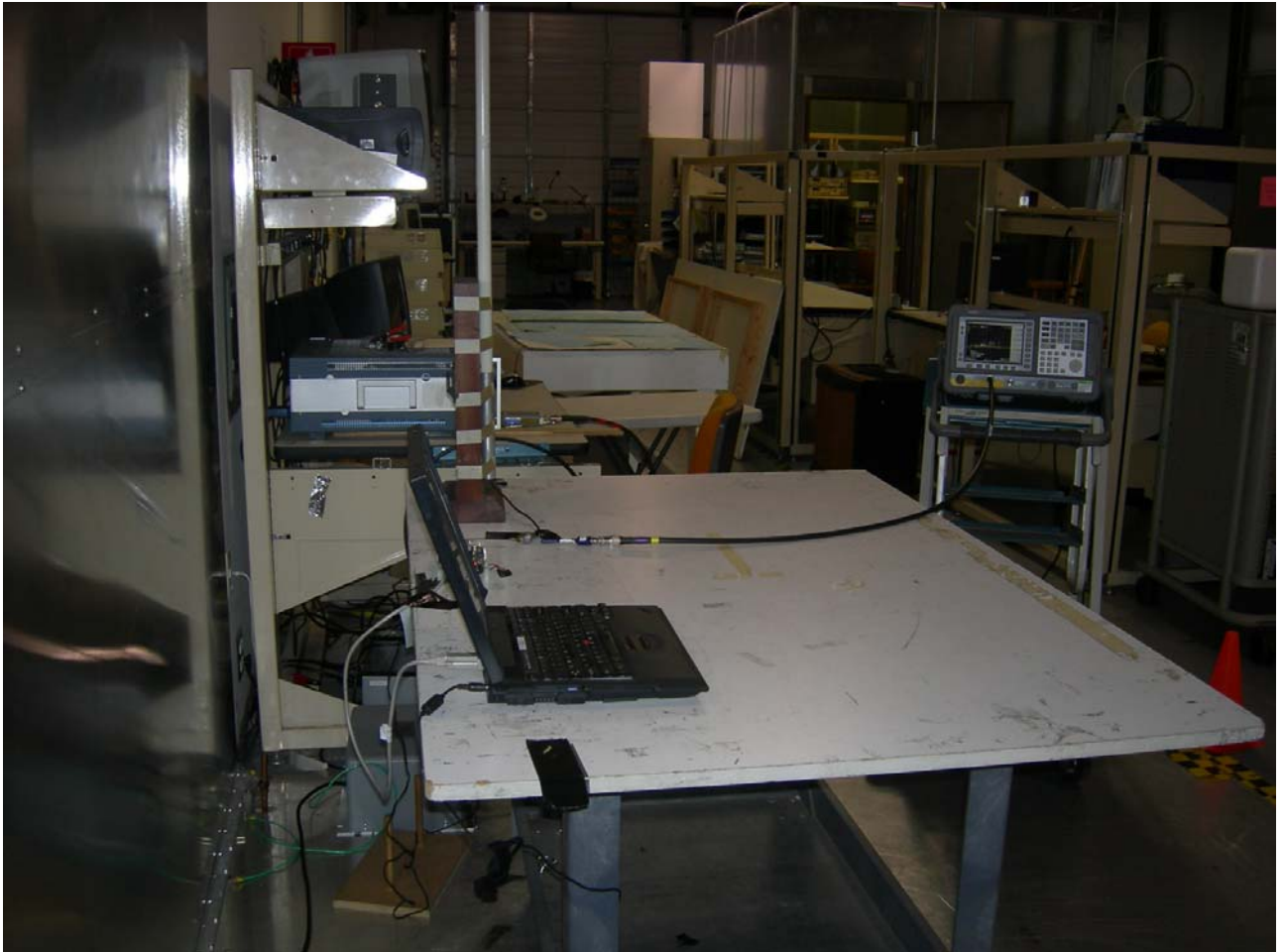
Figure 10: Conducted Emissions Test Set Up – Dipole Antenna
