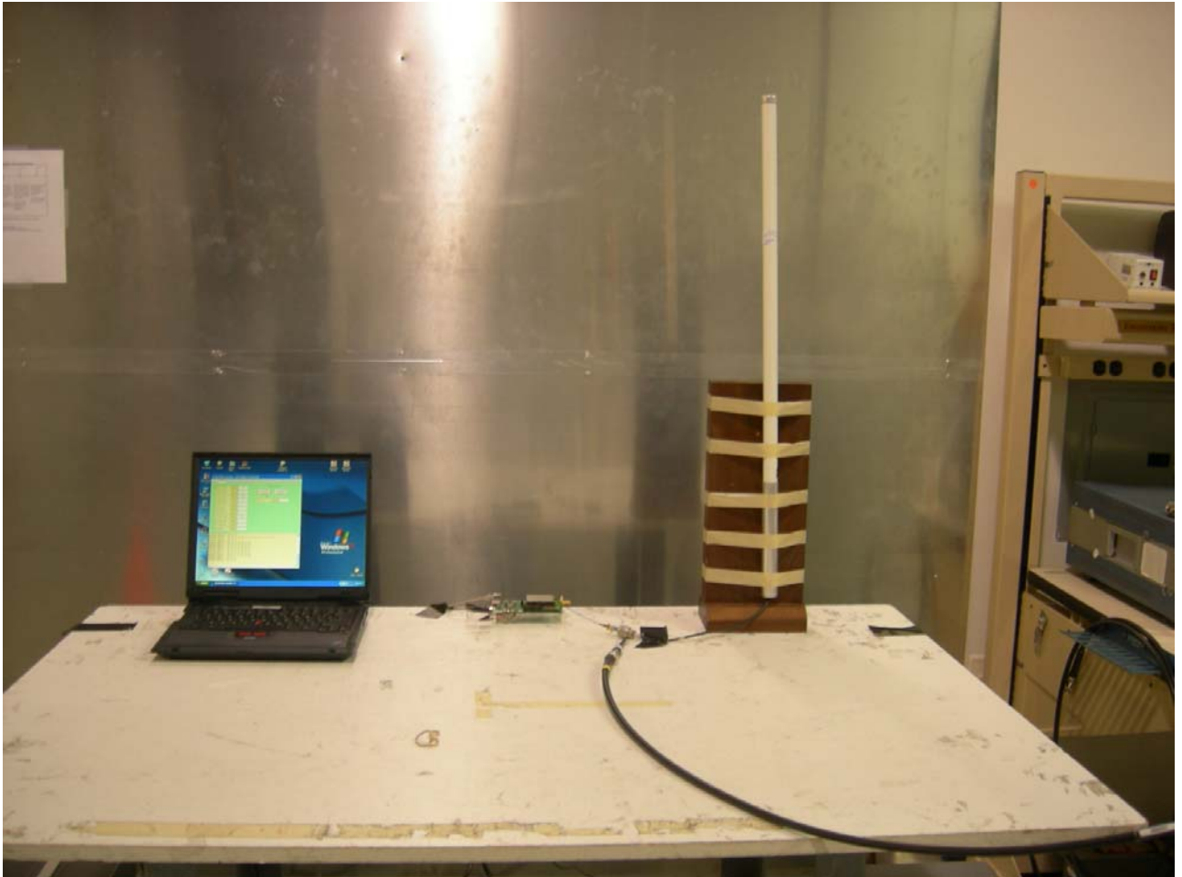
Figure 9: Conducted Emissions Test Set Up – Dipole Antenna
