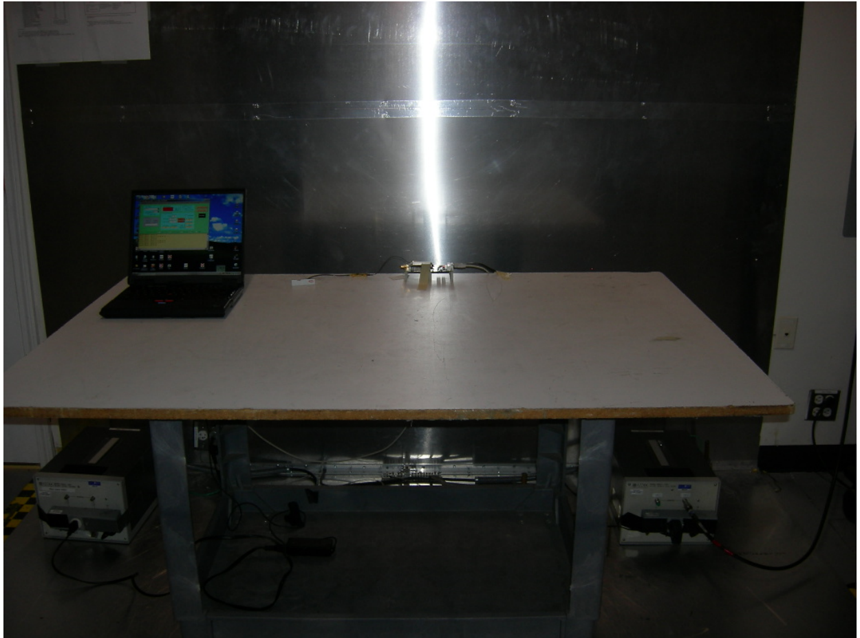
Figure 5: AC Power Line Conducted Emissions – Patch Antenna
