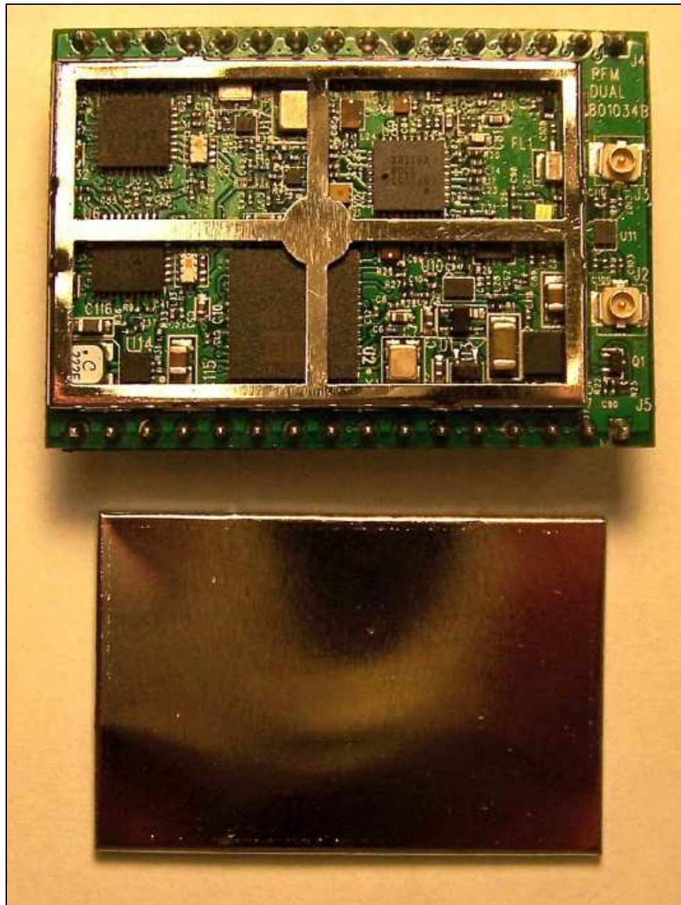
Figure 1: Internal Photo – Shield Removed
