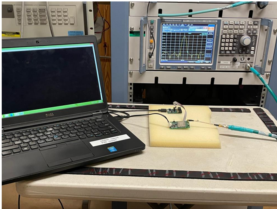
Figure 1: Equipment Under Test – Antenna Port Conducted measurement
