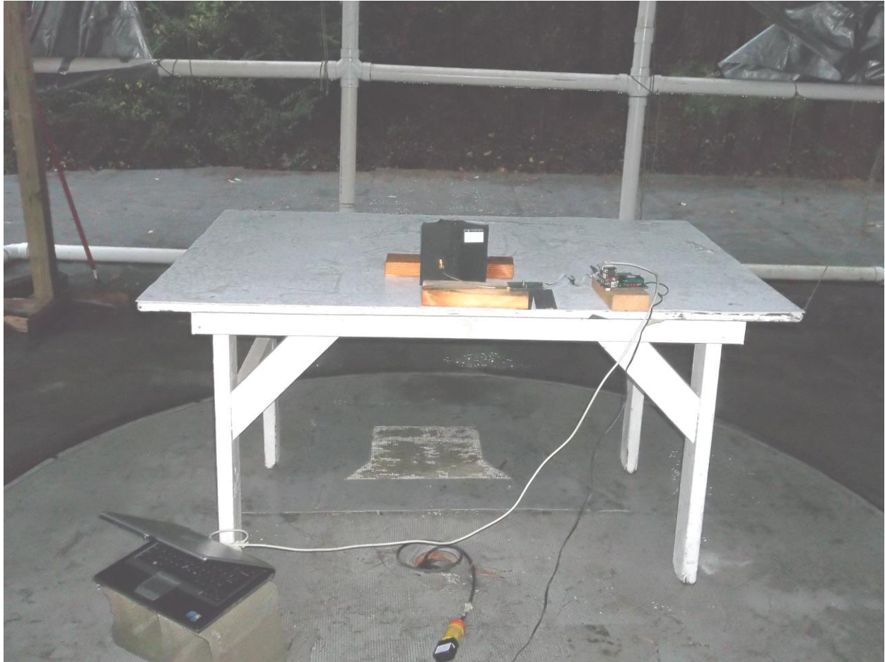
Figure 1. Radiated Emissions Test Setup
