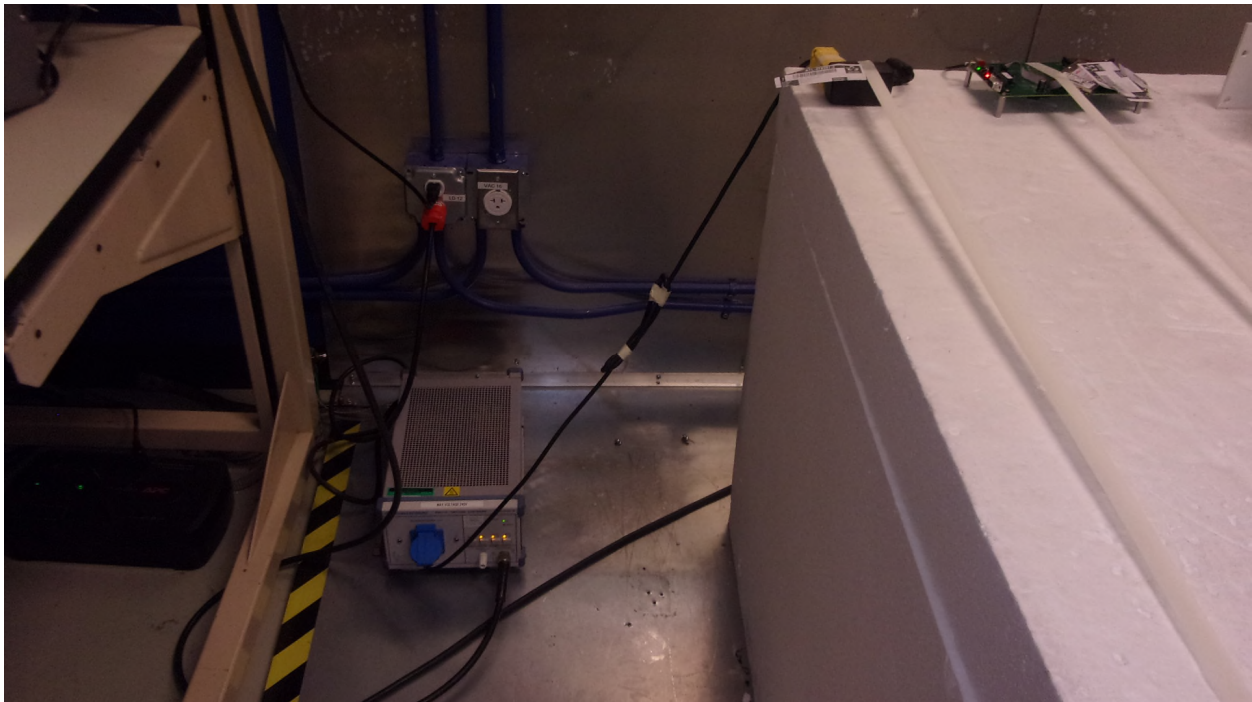
Figure 10: Equipment Under Test – AC Conducted Emissions
