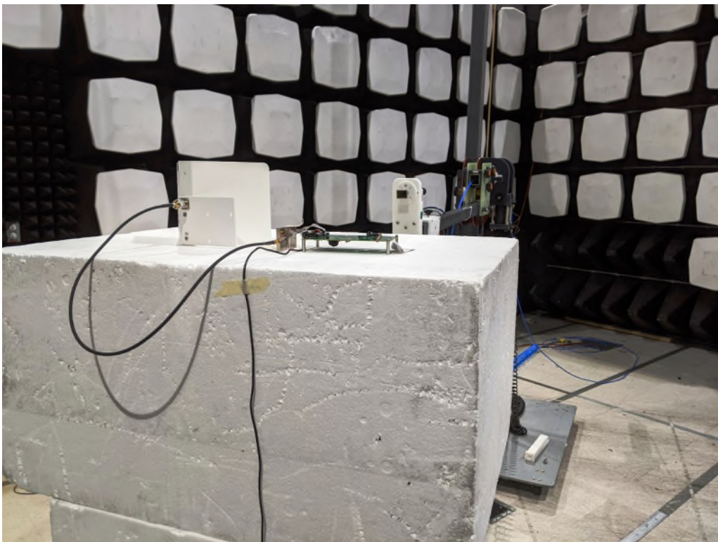
Figure 8: Equipment Under Test – Radiated Emissions – >18GHz
