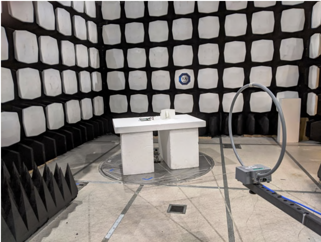
Figure 1: Equipment Under Test – Radiated Emissions – <30MHz
