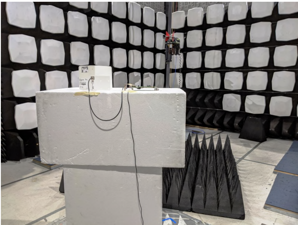
Figure 6: Equipment Under Test – Radiated Emissions – >1GHz
