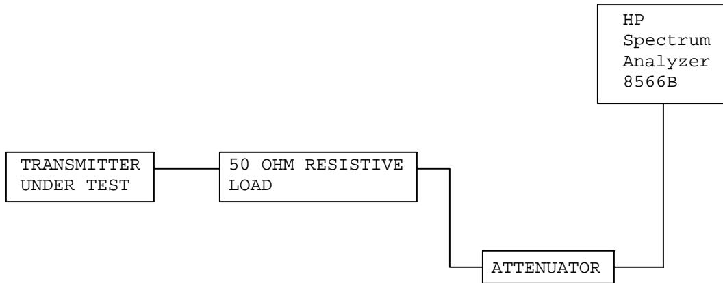
NAME OF TEST: SPURIOUS EMISSIONS AT ANTENNA TERMINALS
