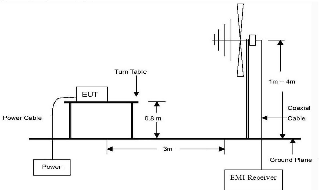
The diagram below shows the test setup that is utilized to make the measurements for emission from 1 GHz to 18 GHz Emissions.
