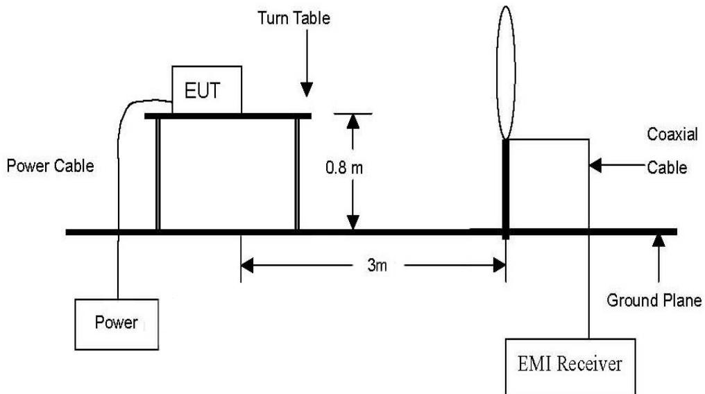
The diagram below shows the test setup that is utilized to make the measurements for emission from 30 MHz to 1 GHz Emissions.
