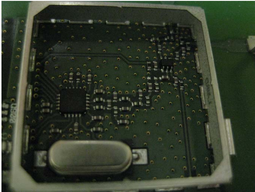
Close-Up of RF Section, Unshielded, View #5
