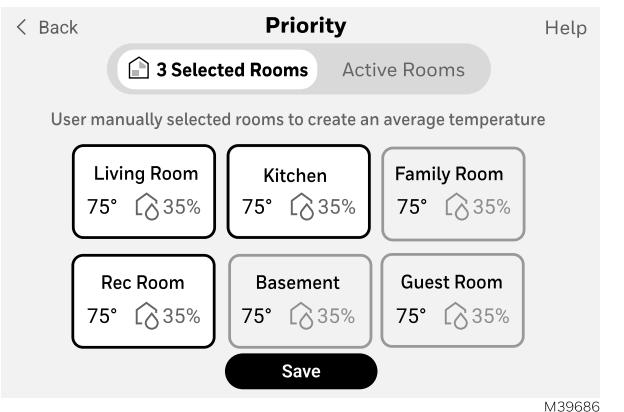
Prioritize different areas of your home by using compatible wireless indoor room sensors. You can manually select these areas or allow the sensors to do it automatically when activity is sensed.
