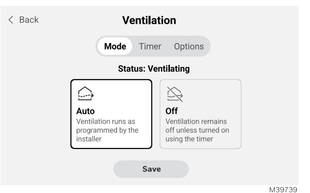
If the thermostat has been set to control Indoor air quality there will be options to control humidity and/or ventilation. Those can easily be adjusted in the user menu on the thermostat or in app.
