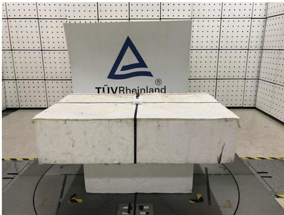
Photograph 1: Set-up for Radiated Emissions (Front View)
