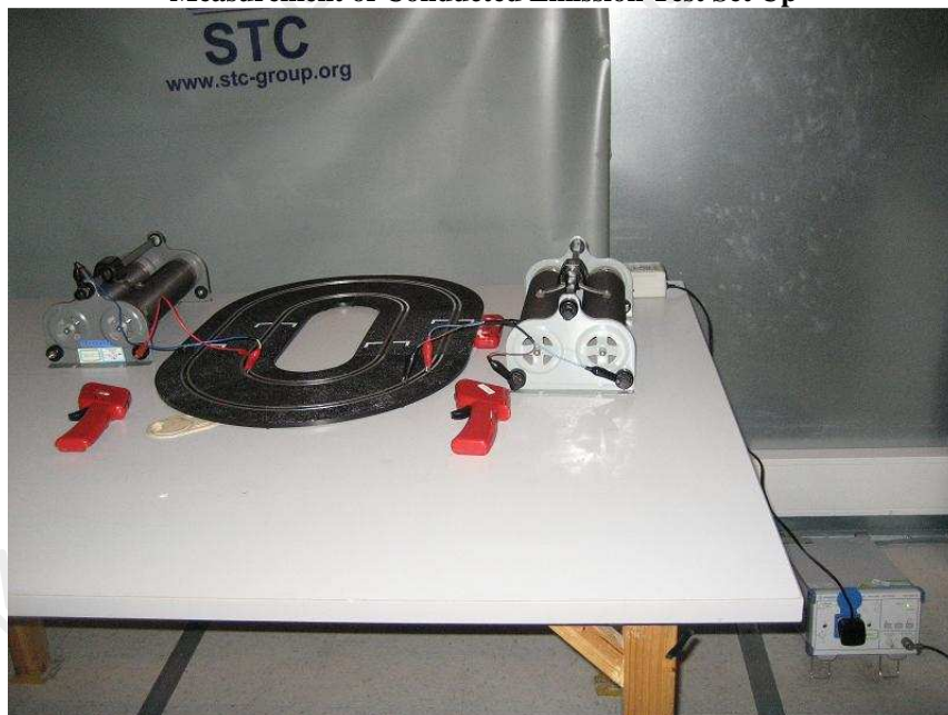
Measurement of Conducted Emission Test Set Up
