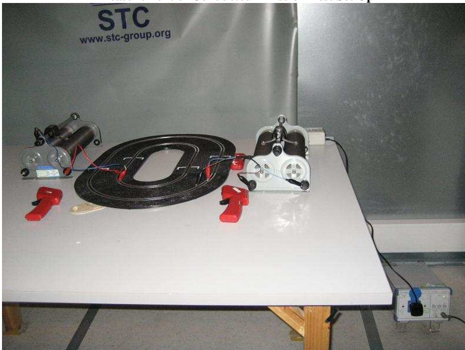
Measurement of Conducted Emission Test Set Up
