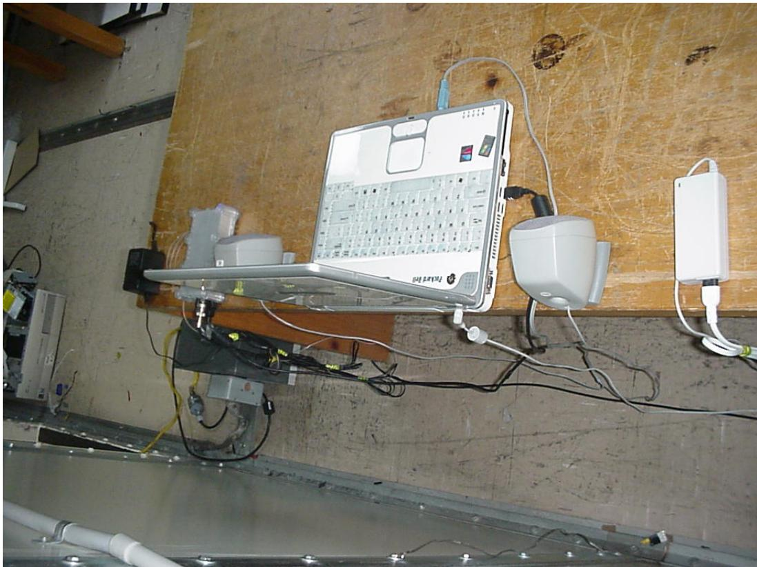
**Radiated Emissions Test Setup**
