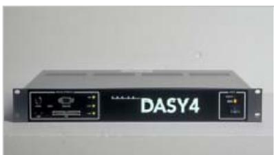
The DASY4 measurement server is based on a PC/104 CPU board with a 166MHz low-power Pentium, 32MB chip disk and 64MB RAM. The necessary circuits for communication with either the DAE3 electronic box as well as the 16-bit AD-converter system for optical detection and digital I/O interface are contained on the DASY4 I/O-board, which is directly connected to the PC/104 bus of the CPU board.
