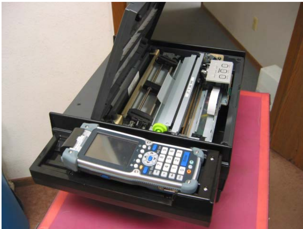
6820 Printer with paper loading door open
