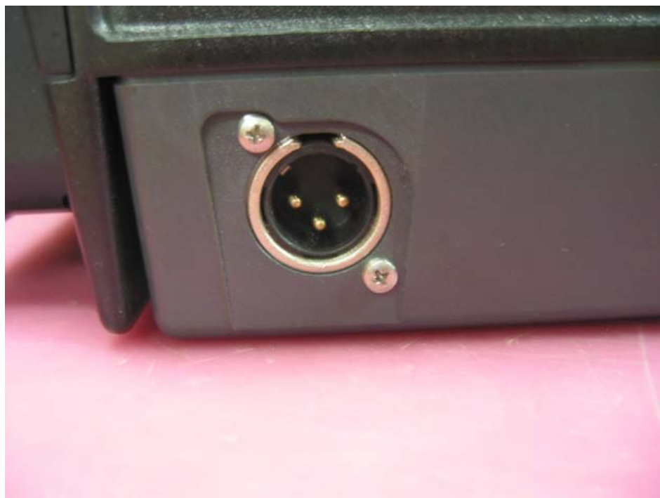
Close-up of DC Power Input
