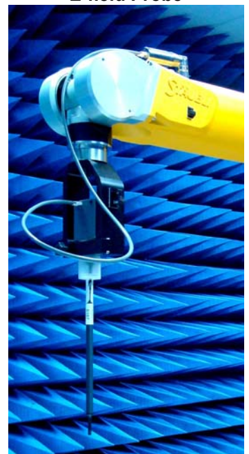
Figure 7. Probe setup on robot
