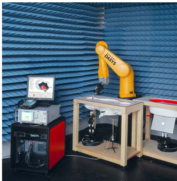
Fig. 5.2 Probe Setup on Robot
