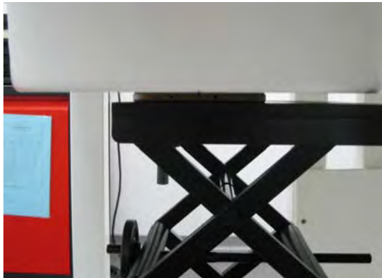
Fig.3 EUT Lap-held mode to flat phantom
