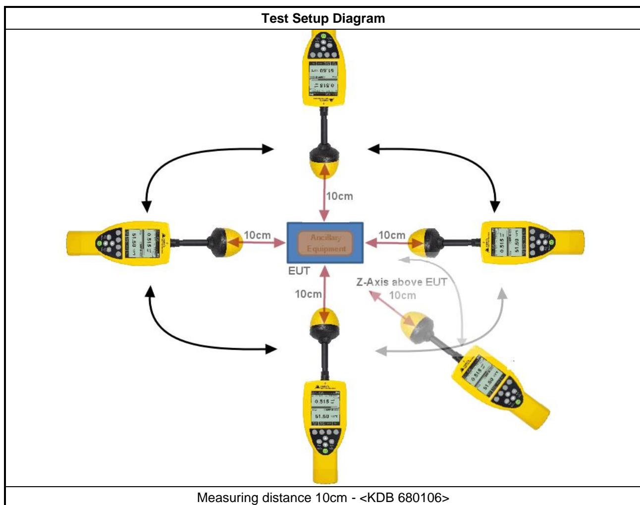
**Test Setup of H-Field**
