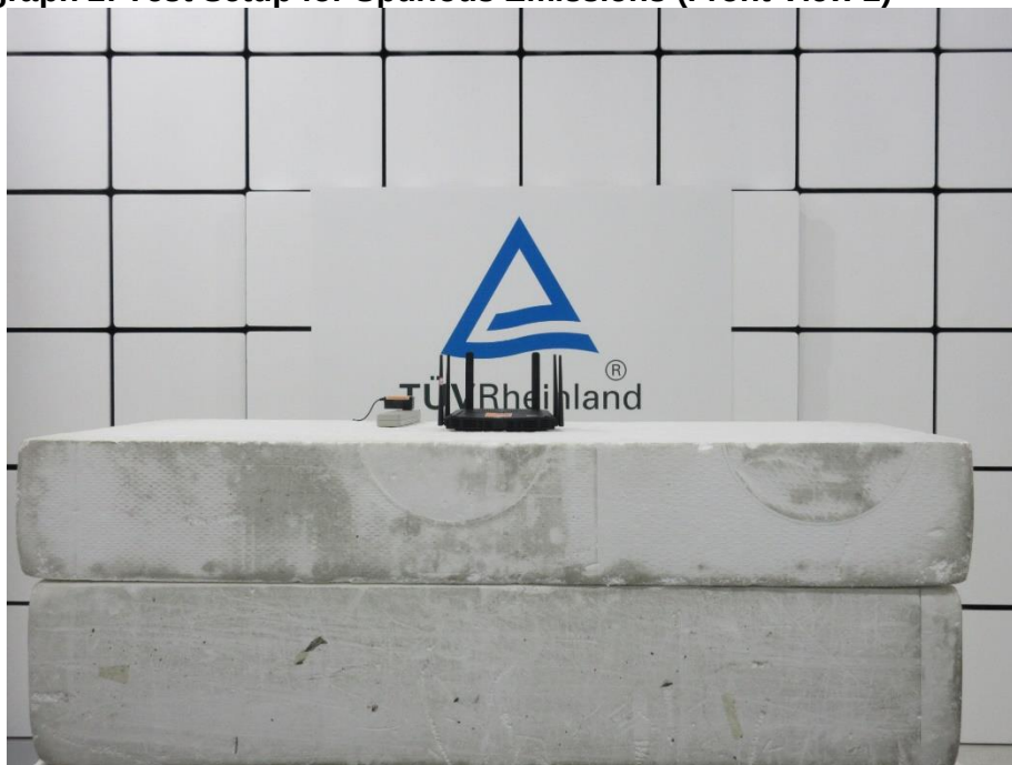
Photograph 2: Test Setup for Spurious Emissions (Front View 2)
