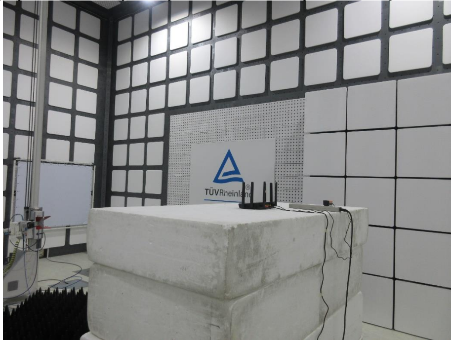
Photograph 6: Test Setup for Spurious Emissions (Back View 4)
