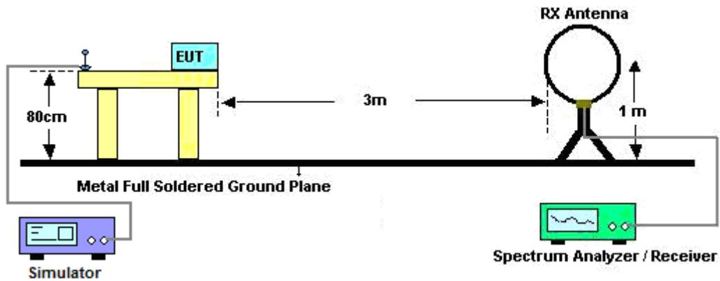
For radiated emissions from 30MHz to 1GHz
