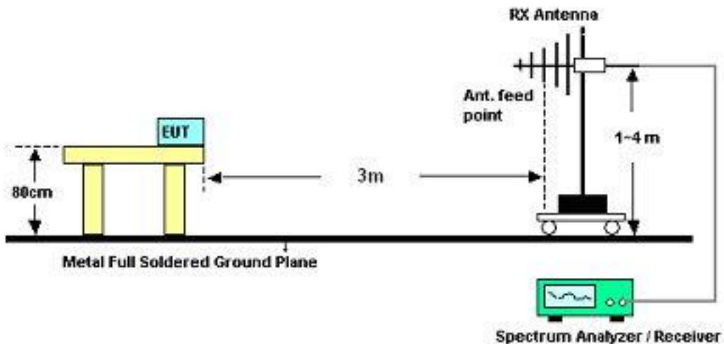
**For radiated emissions above 1GHz**
