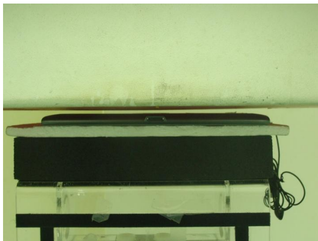
Rear Face of the DUT with earphone for Phantom 0.5 cm Gap with Sample 2
