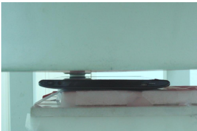
Front Face of the DUT with Phantom 10 mm Gap (Voluntarily submitted)
