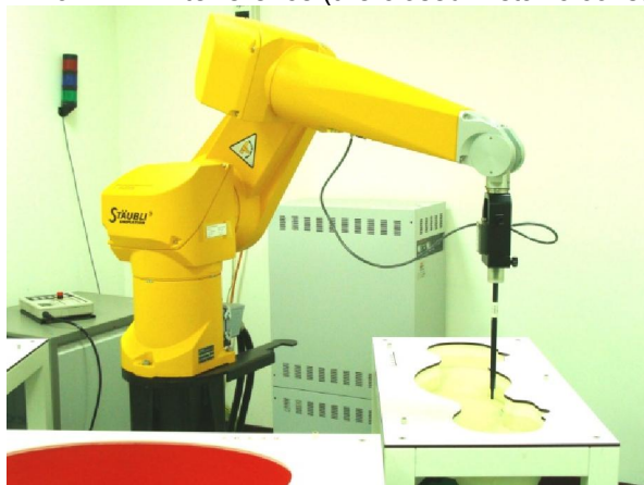
Fig 5.5 Photo of DASY4
