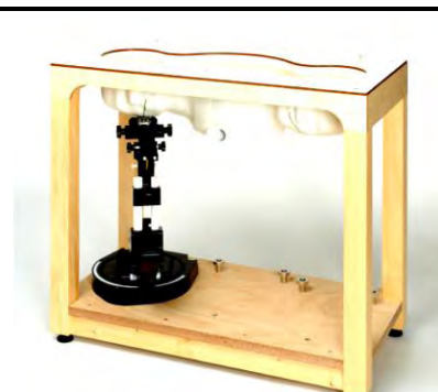
Fig 5.9 Photo of SAM Phantom
