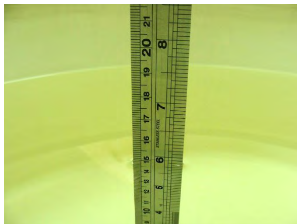
Fig 6.2 Photo of Liquid Height for Body SAR
