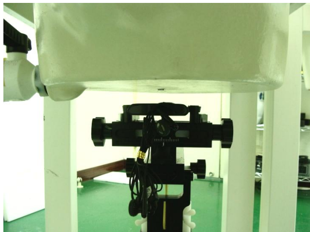
Bottom of the DUT with Phantom 1.5 cm Gap with Earphone 2 for Sample A
