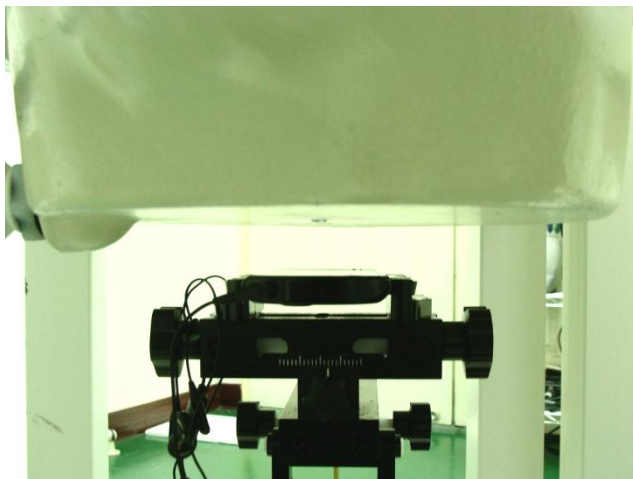
Face of the DUT with Phantom 2.5 cm Gap with Earphone 1 for Sample B
