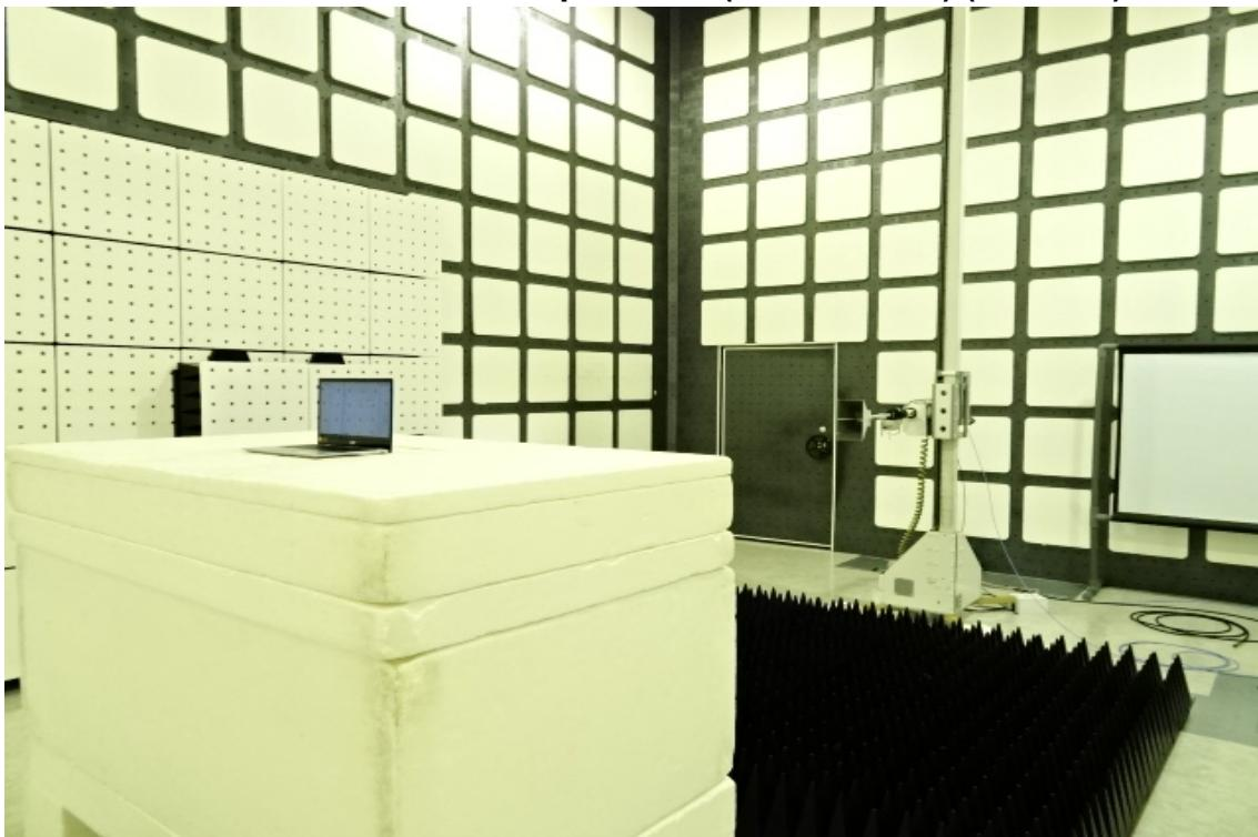
**Radiated Emission Set up Photos (Front View)**
