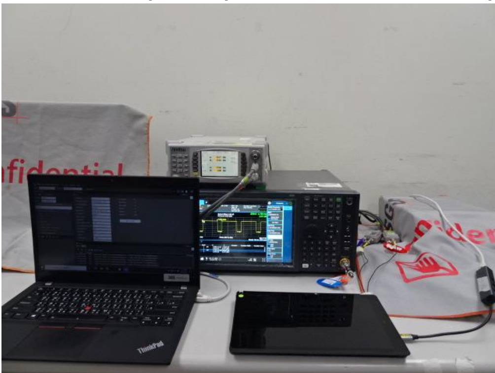
Conducted Setup Photo (Measurement at Antenna Port)
