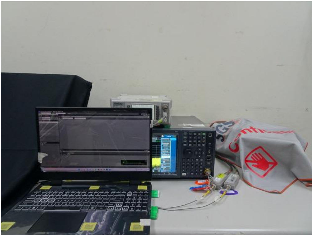
Conducted Setup Photo (Measurement at Antenna Port)
