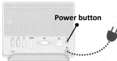
2. **Wait until the LED light on the front panel blinks in amber** to indicate the Dock is standing by and ready to be connected.
