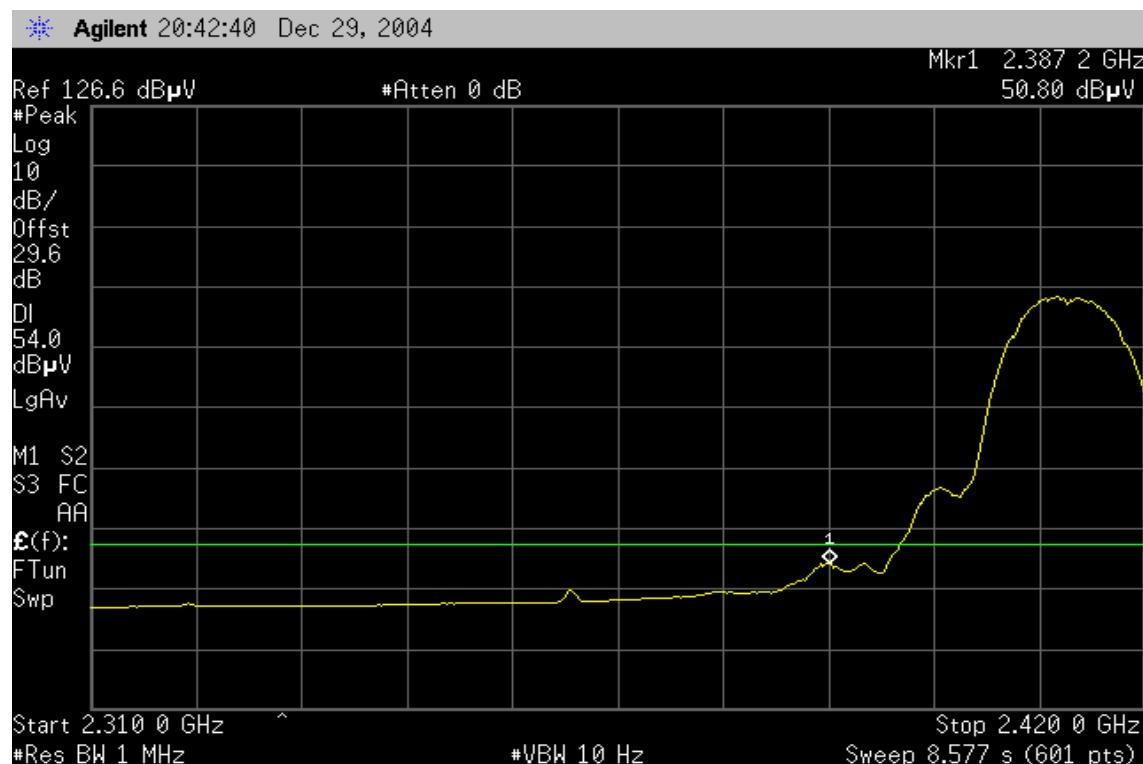
**Band Edges (IEEE 802.11b / CH High)****Detector mode: Peak****Polarity: Vertical**
