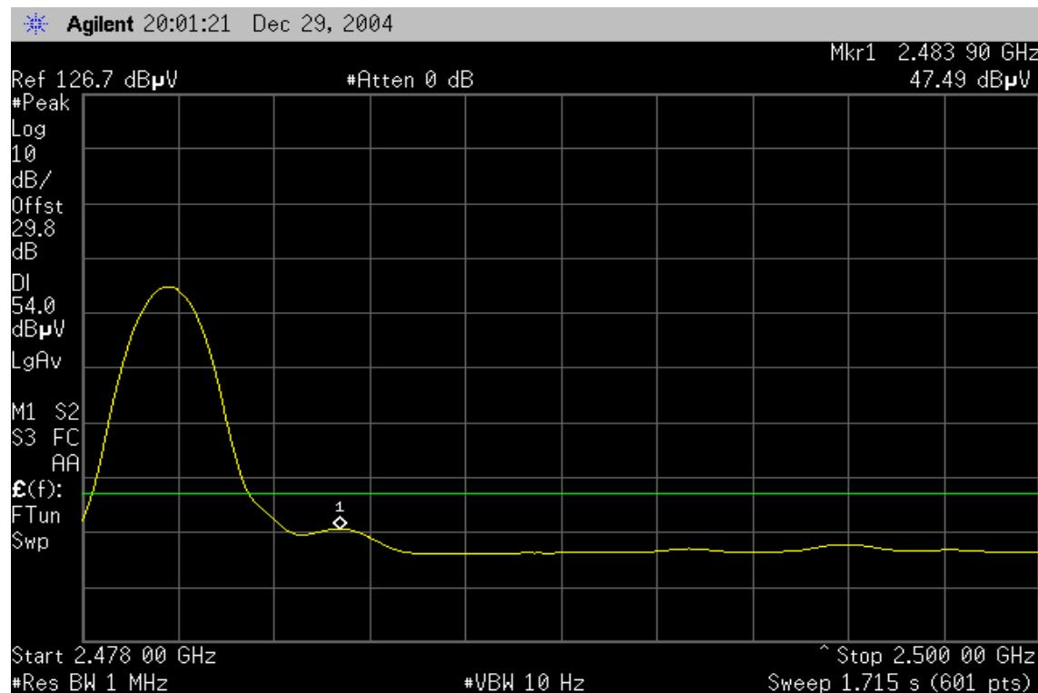
**Detector mode: Peak****Polarity: Horizontal**
