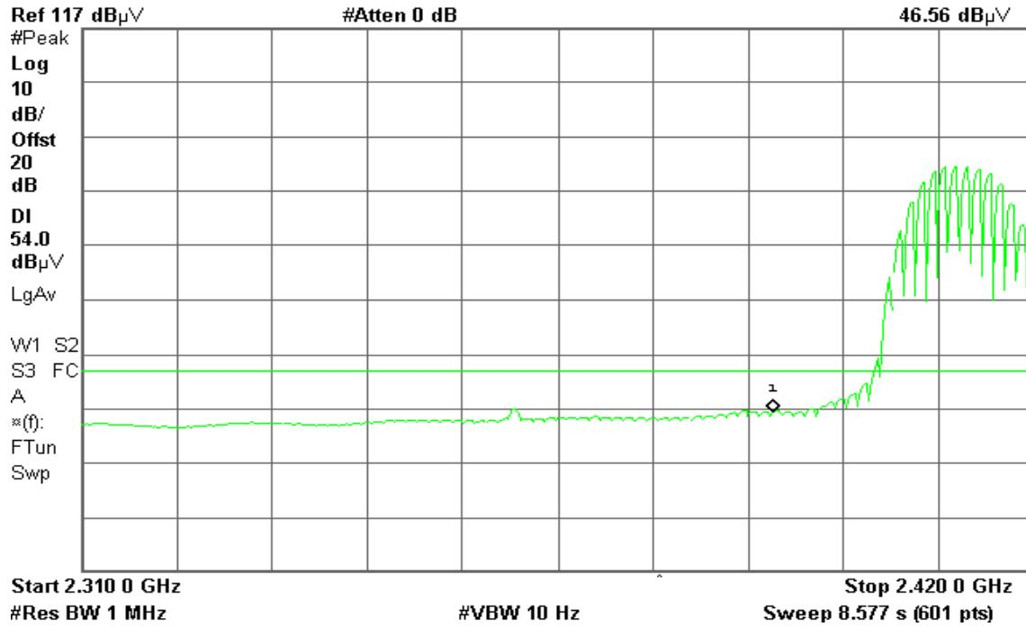
**Band Edges (WLAN TX Mode / CH High + BT TX Mode / CH Mid)****Detector mode: Peak****Polarity: Vertical**
