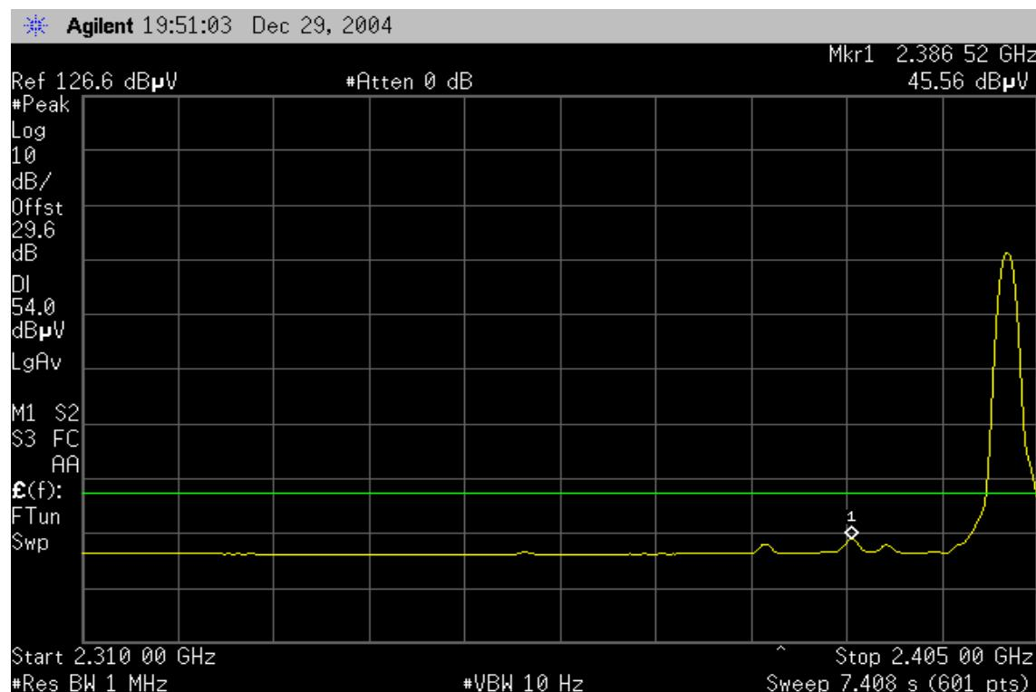
**Band Edges (Bluetooth / CH-High)****Detector mode: Peak****Polarity: Vertical**
