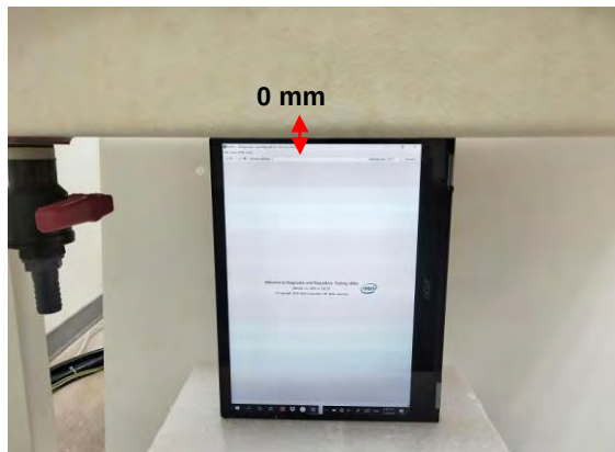
Fig.6 EUT Right side to flat phantom
