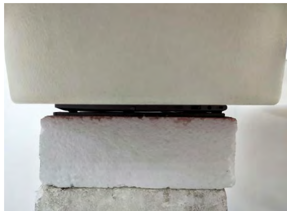
Fig.3 EUT Back side to flat phantom
