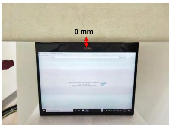
Fig.5 EUT Bottom side to flat phantom
